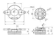
Includes one winding plug and one stationary plug. Centre distance of mounting holes: 136-138 mm. The winding plug has two 3/8" set screws for fixing to the shaft. Stationary plug has a 50,8 mm hole for bearing placement. Max. Torque:157Nm. Suitable for 1 inch (25,4mm) shaft. Max torque bolts 20Nm. Unit:Pair (Stationary plug (S) + Winding plug (W))Weight:0.61 kg / prMaterial:AluminiumThread:Universal L+R, max. 10mm.Marking:None.
